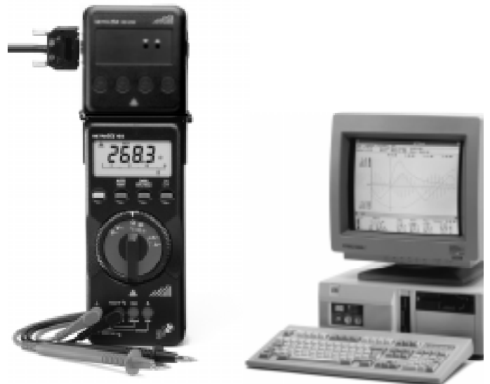
PC with METRAwin10 and digital multimeter with BD232 interface adapter
